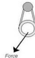
Spinning rods and spiral wrapped rods have guides on the bottom of the rod, therefore they do not twist, because there is no torque (turning moment) applied to the rod's tip top
